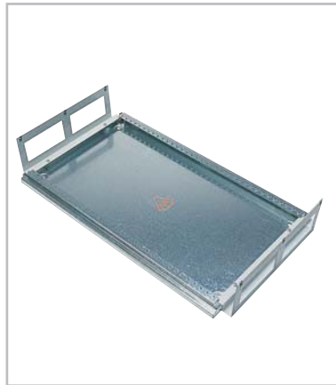
The 1.5 mm thick steel rear panel is equipped with 8 mm diameter holes at distances of 25 mm. The sendzimir zinc plated steel, which complies with EMC regulations, ensures improved earthing.
