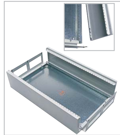
An ingenious system of grooves makes it possible to fix the side panels on the rear panel without screws being needed.
